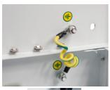
Before fitting the front cover, ensure that the earth bond is connected between the enclosure base and the front cover. To relieve undue pressure on the stud, first fit the M6 plain nut and washer. Fit the earth cable to the stud, and secure using the nylok nut; by locking the two nuts against each other.
